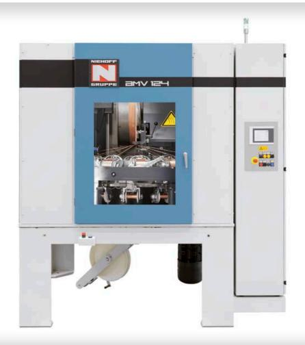
**BMV 124** Rotary Braiding Machine with 24 bobbins
