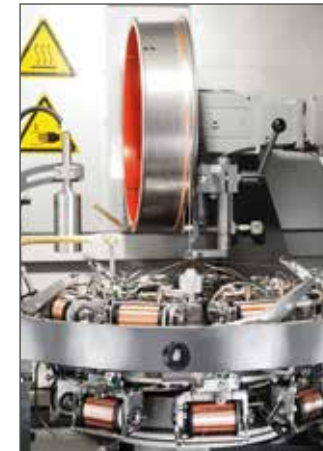
bobbin carrier with tension control (max. spool size 80 x 100/80 mm)
