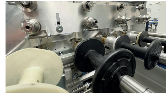
SMB 4: automatic wire winding machine with 4 spindles
